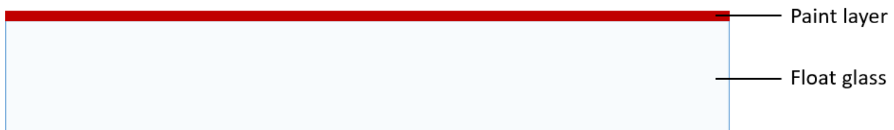
Figure 1: Schematic diagram of the composition of a Lacobel
